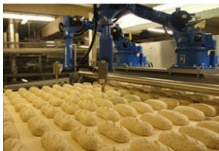
Automotive, high productivity dough pieces' cutting with Gostol 'ROBO CUT' equipment in production in bakery in Norway
